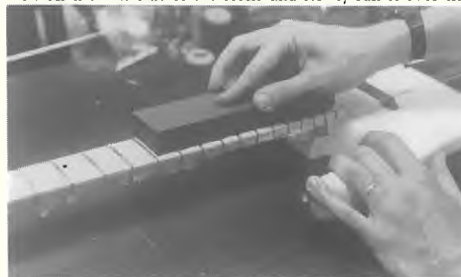
Stoning the frets - note masking tape protecting fretboard
