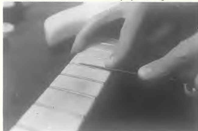
Profiling the fret with a knife-taper needle file
