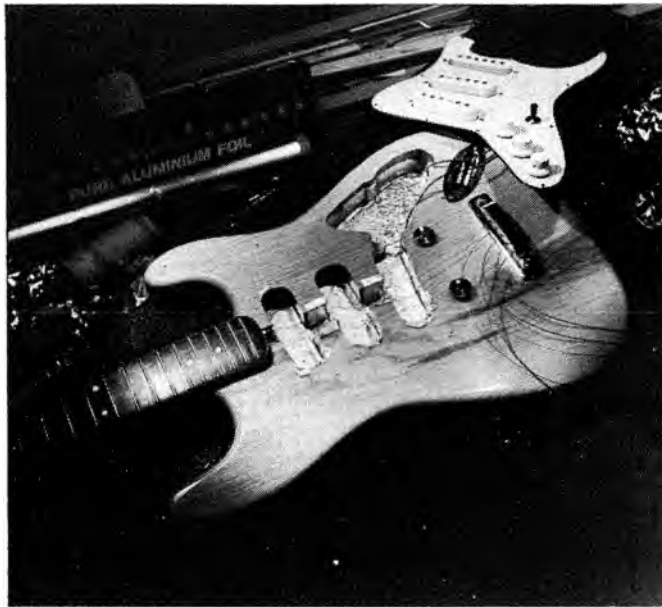
Cavities lined with foil, note overlapping tabs
