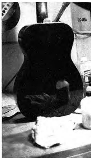
Mirror finish of original lacquer, after restoration
