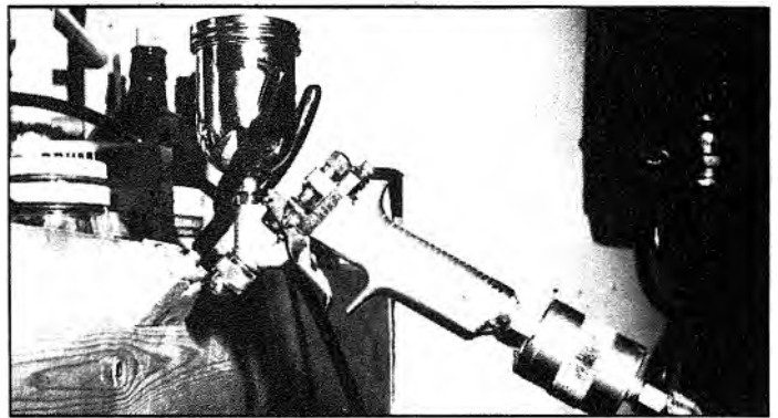
De Vilbiss MP Gun. The support fork is set at an angle to the wall to keep the cup upright when not in use. Note the filter attached between the airline and the gun.
