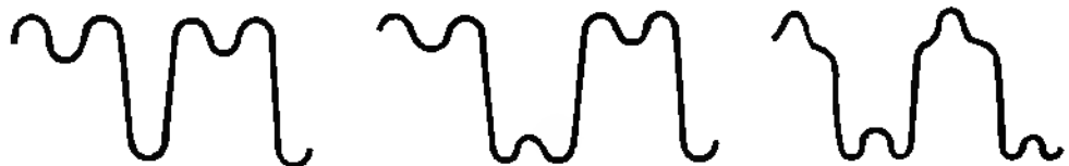
Simple distortion patterns obtained in an audio amp.
