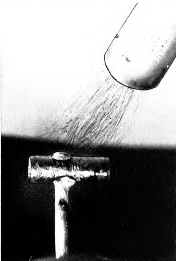
At bright red, the solder "runs" and looks like this.
