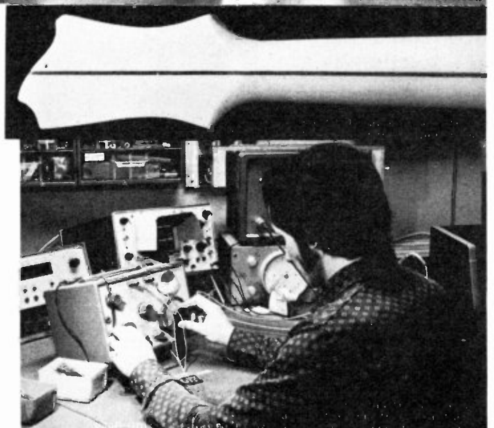
The shapes of things to come. This is the neck of the Superswede. Notice the Schaller machine heads, the butted neck and the rounded heel.
