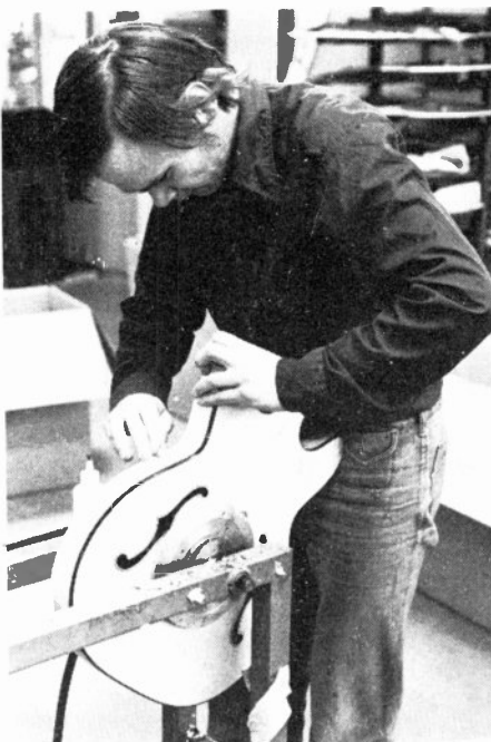
Each Hagstrom solid guitar receives two coats of Polyester finish. Each guitar is hand scraped between coats to ensure a really fantastic finish.
