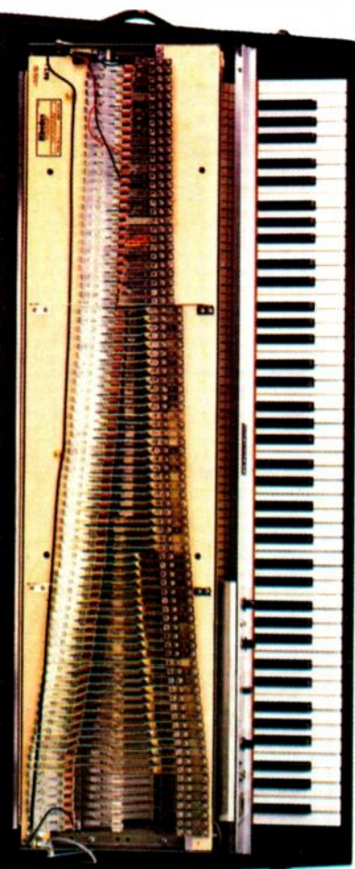
Pitch, volume and timbre are all easily adjusted in the harp assembly. Tuning fork, one bars, tuning springs and pickups are all adjustable.
