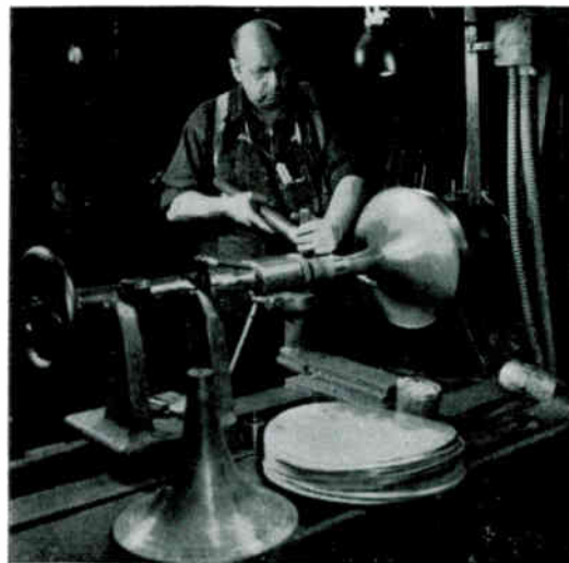
Conn craftsman spins a French horn bell from a flat disc of brass.
