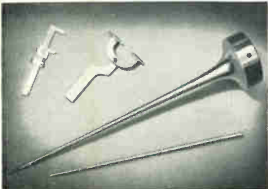
Photo of actual master steel mandrels used to form the famous 22B mouthpipe and bell. These two mandrels are priceless, representing the accumulated experience of years of trumpet making.
