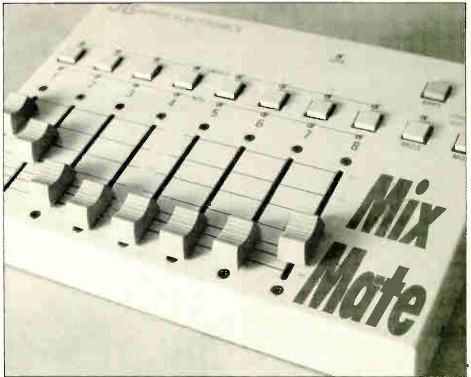
– **Normal/Read All:** This is the Playback mode where Mix Mate re-enacts the previously recorded fader and mute moves while locked to incoming sync. New fader and mute moves are not recorded, as the memory is protected in this mode.
