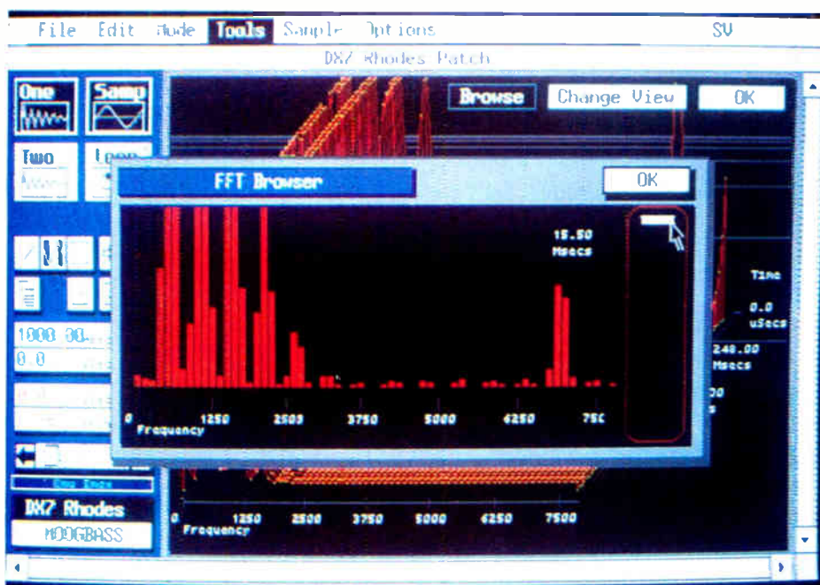
The FFT Browser function allows you to dissect a waveform and see how it changes over time.
