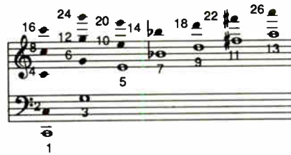
Figure 8. The Coarse Frequency Ratio numbers, which step you through the overtone series, are easily memorized as a dominant 13th chord with a sharp 11th. In the voicing shown below it's the whole notes: 1, 3, 5, 7, 9, 11, 13 (all odd numbers). Any even numbers can simply be divided in half until a familiar odd number appears. Each division by two means that you've descended in pitch by one octave. This system also works for the harmonic overtones of the sawtooth, where all odd and even numbers are present, and for the square wave, where there are no even numbers (no octave duplications).
