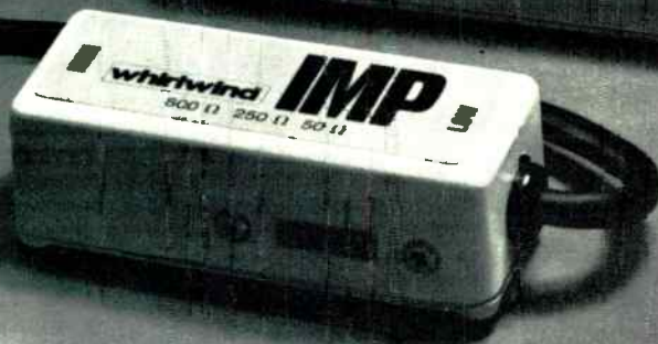
IMP: Converts from high to low, and vice versa. A three-way slice switch lets you choose between 50, 250, or 600-ohm conversions.
