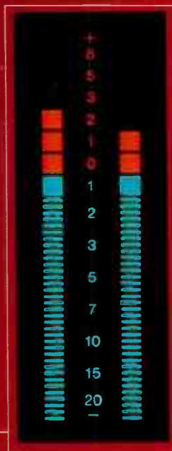
Large, fluorescent, high intensity bargraph peak meters
