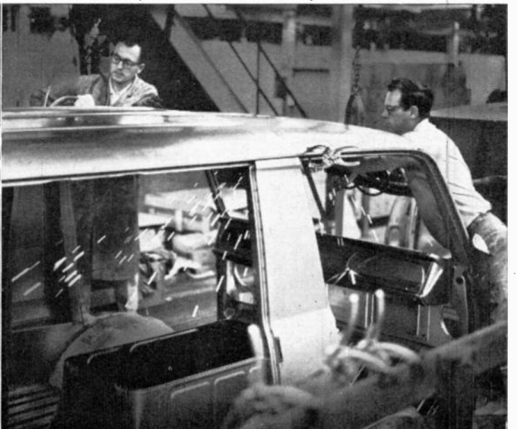
followed by front end panels, many galvanized... and a ribbed roof panel caps the structure.
