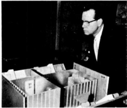
COVER: Room ambient calorimeter at Electrical Testing Laboratories, N. Y., is used for NEMA room air conditioner certification program. Shown is Hoffman S. Beagle, ETL president. See story on page 29.
