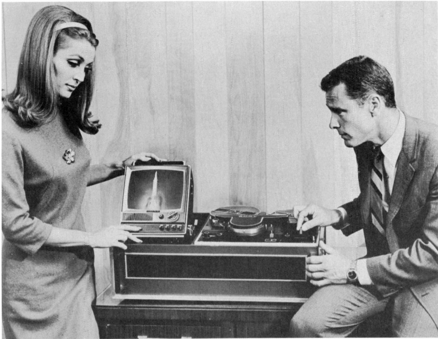
SONY "VIDEORECORDER," fully transistorized home video tape recorder, priced at $995, is scheduled to be marketed in U. S. by first week in August. Weighing 66 pounds, unit uses one-half-inch wide tape that moves at 7½ inches per second. Video camera kit, available as optional equipment, permits recording family pictures in black and white with sound and showing them immediately on nine-inch screen.
