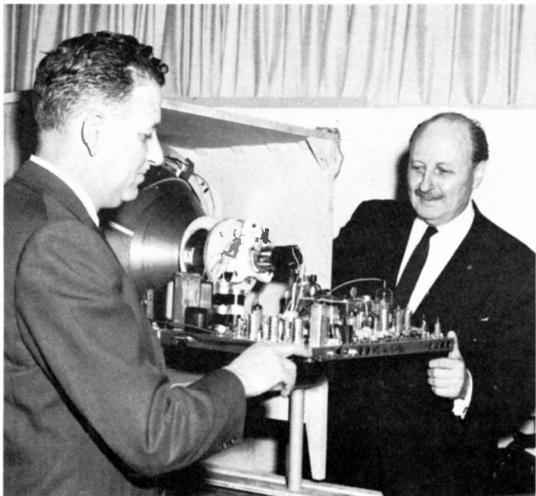
COLOR CHASSIS developed by Electrohome is inspected by Carl A. Pollock (right), president, and Howard W. Main, vice president. Chassis has swing-down feature for easy servicing.
