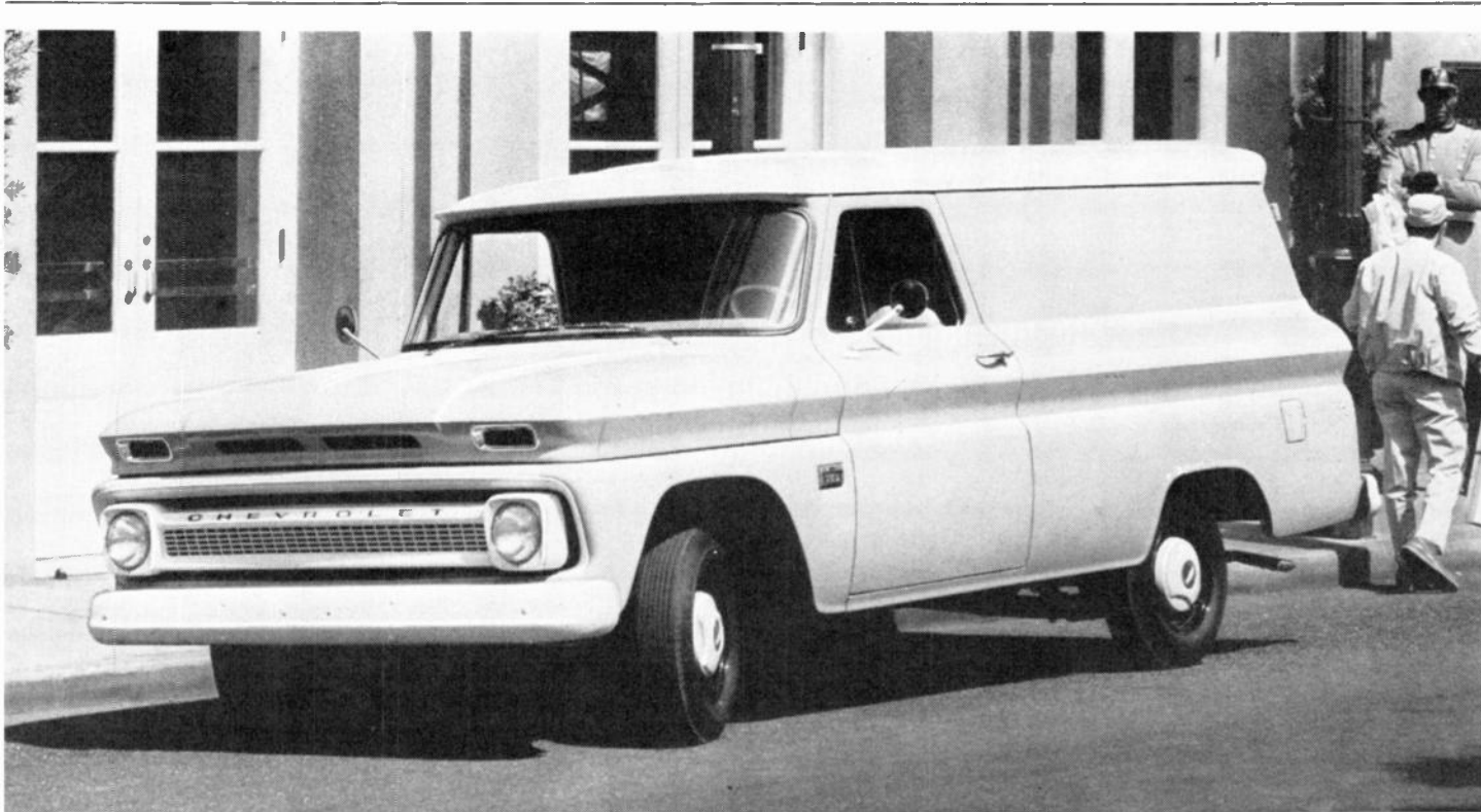
PANELS —Select either the ½-ton model with 7½-ft. body or the extra-long 1-ton model with 10½-ft. body. You can even have 4-wheel drive with the 7½-ft. body. All models feature smooth laminated wood floors with full-length steel skid strips for easy cargo handling.
