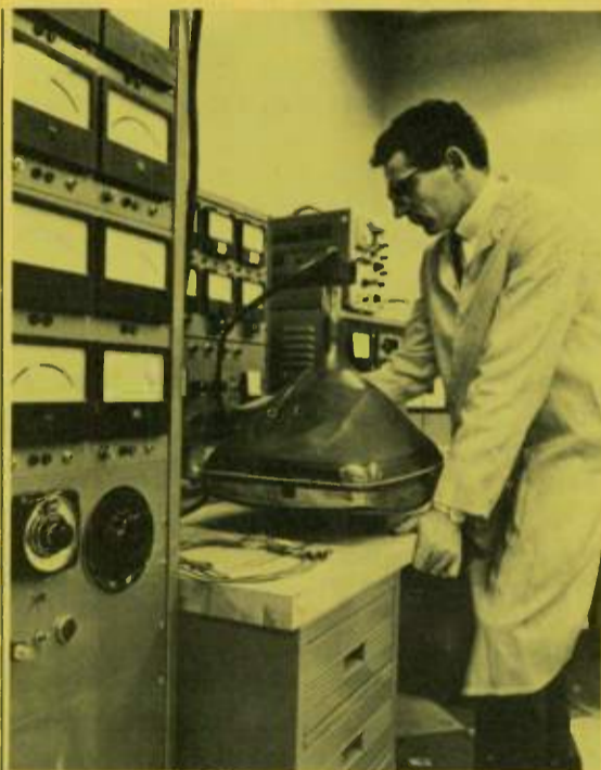
Admiral color tube technician checks 23-in. picture tube. Part of inspection is the "aging" of tri-gun assembly which is conducted by applying current to the filaments of assembly.
