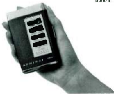
Sonar full-function 7-button Remote Control, available with many models. Turns set on and off, adjusts color intensity, tint, changes channels and adjusts volume.
