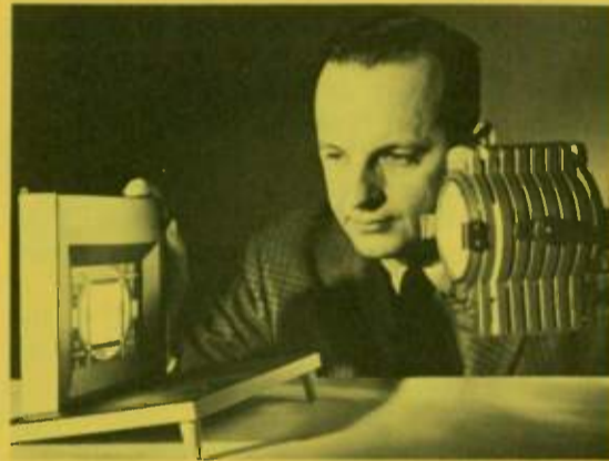
The brighter the better: Dr. George Heilmeier demonstrates RCA's new high-resolution liquid crystal display whose images are seen by reflection and, therefore, grow stronger as the light shining on them grows brighter. This contrasts with most electronically controlled displays, such as TV tubes, which "wash out" under bright light.
