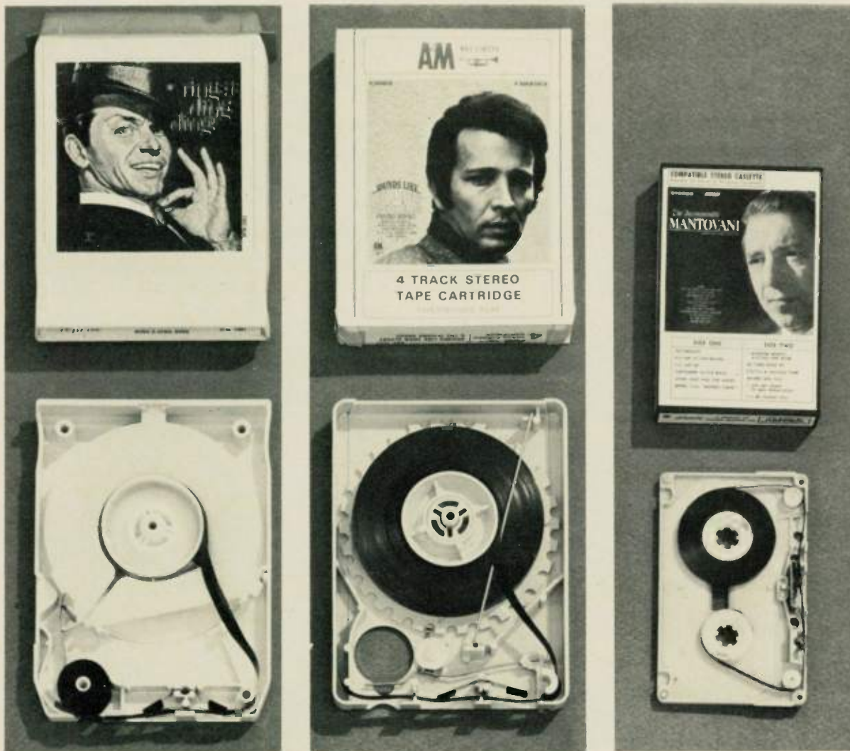
Cutaway views show relative size and complexity of two cartridge systems and cassette. Shown (1. to r.) are Lear eight-track cartridge, four-track "Fidelipac," and Philips cassette.
