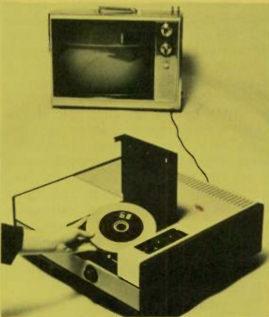
Placing EVR film cartridge in position for sight and sound transmission on conventional TV set.
