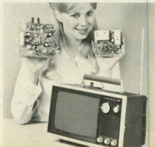
The first all-transistor TV set offered by Admiral is the 12-lb. "Travel Mate" with 26 transistors and 18 diodes. It can be played anywhere by using an optional 12-volt power pack and charger. It has an open list price.
