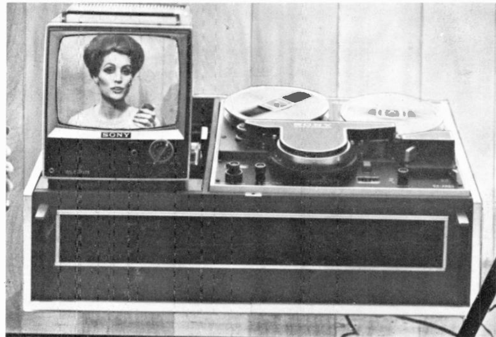
Sony's $995 home video tape recorder; records for 60 minutes on a 7-inch reel
