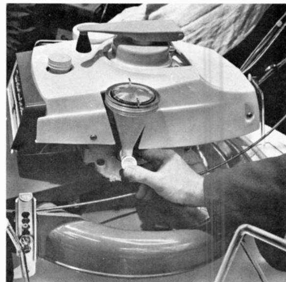
An easily viewed oil gauge, and edge-trimmer are two new features in Toro's mower line
