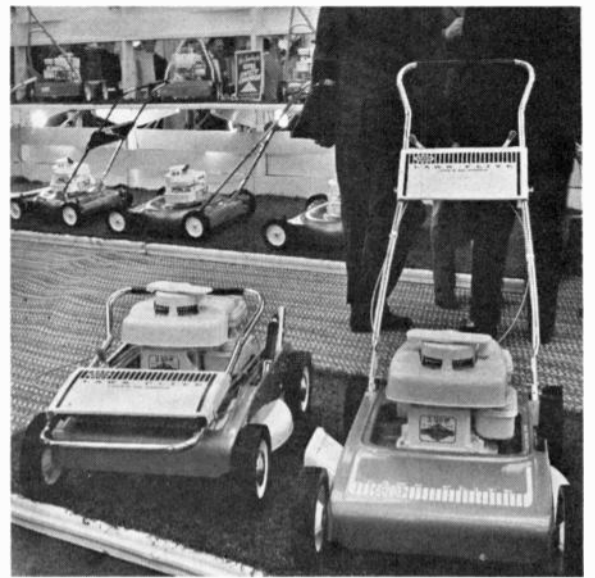
MTD's folding handle, seen here in both positions, is a potential space saver
