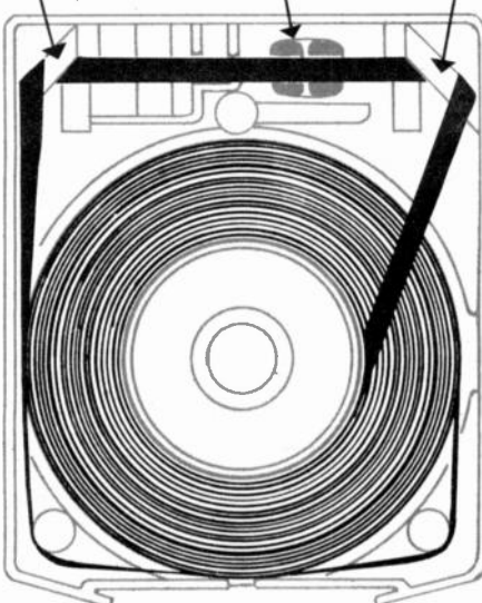
Orrtronic cartridge —Tape exits at a 90 degree angle to the rest of the spool and passes over the player head in a horizontal position. This drawing shows player head.
