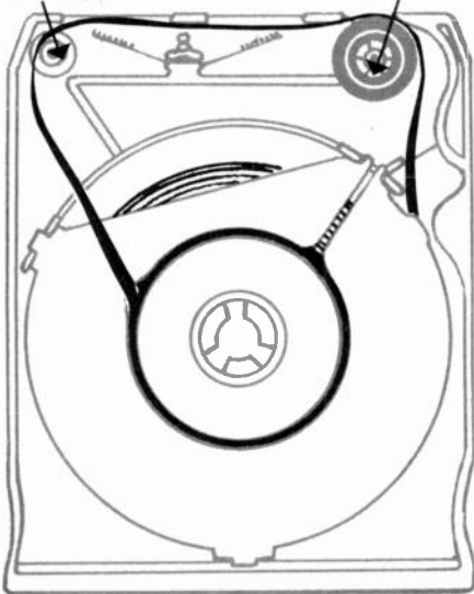
Lear cartridge —As in Fidelipac, tape exits from inner hub, is taken up on the outer edge. But here, pinch roller to advance tape is in the cartridge itself.
