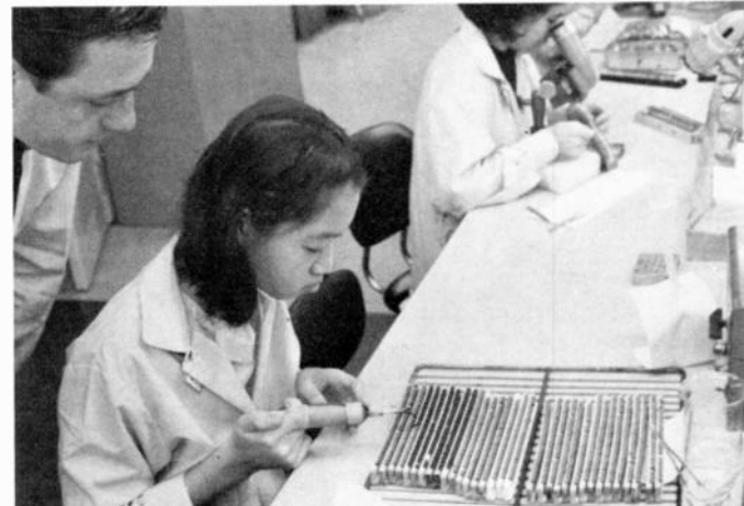
At Semiconductor Ltd., a girl applies a drop of epoxy resin to the top of the transistor package to form a seal. This is one of the last steps in the transistor assembly at the Hong Kong plant.
