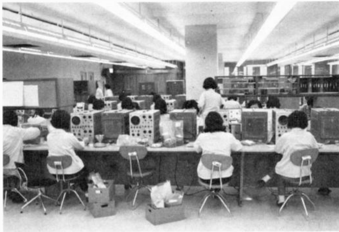
Testing the transistors at Semiconductor is done with oscilloscopes. Note the plastic bags at the girls' feet. Rather than count the number of transistors in a shipment, the company weighs them in these bags.
