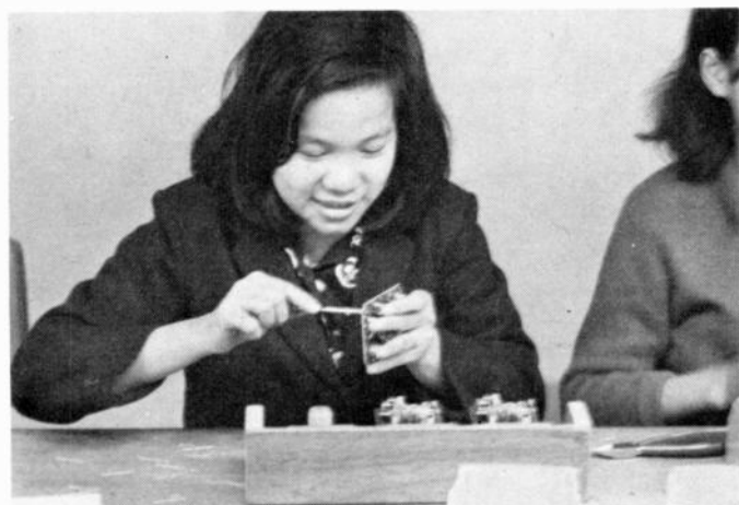
At Transelectronics Ltd.—a joint venture of Zenith and ITT—the assembly line is built so that three radio chassis are mounted on a single carrier—a labor-saving technique the company borrowed from Zenith.
