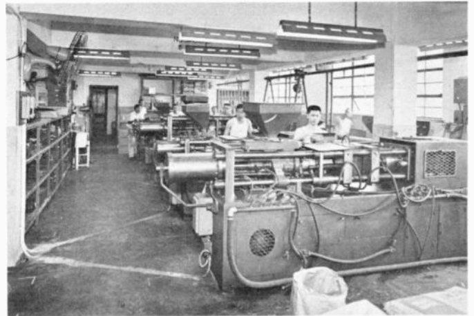
Cabinet molding machines at Trans-World Electronics are part of the company's component fabrication lines. The company, which turned out 1 million radios last year, also builds grilles and printed circuit boards.
