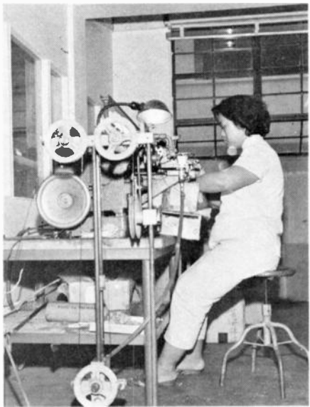
Working at the new Semiconductor building, a girl cuts lead wires on the assembly line. Semiconductor actually assembles transistors, rather than make them. Its starting material is silicon wafers, on each of which several hundred transistors have been fabricated by Fairchild in the U.S. Most of the completed transistors go back to the U.S.
