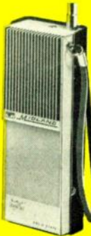
NEW! Micro-Size 11 transistor 100 mw unit just 1" x 1 7/8" x 5 1/4". Only 10 1/2 oz. incl. 9-volt battery. Has chrome die-cast front and battery condition meter. Model 13-125
