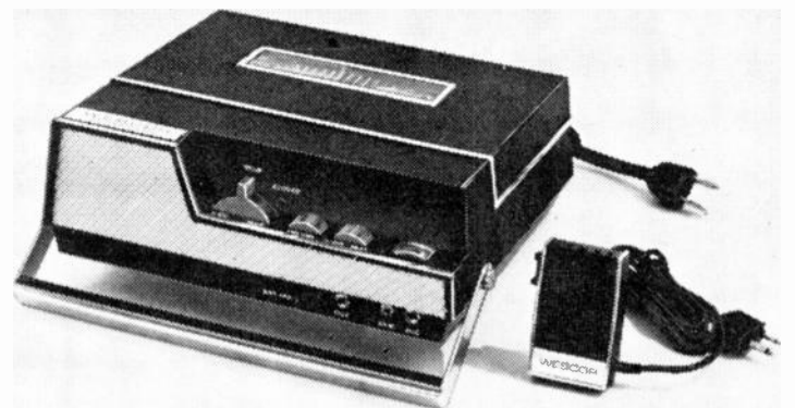
Webcor Rechargeable III—Model 2714: Minimum 800 hours playing time. Recharge overnight. 2 speeds 1½, 3¾. Transistorized capstan speed control. 3" reel, built in AC converter, charger. Operates on 110V, AC, 3 rechargeable batteries (included) or 4 regular flashlight batteries. Combination VU/battery charge meter. Storage compartment holds remote control dynamic microphone, patch cord, earphone.
