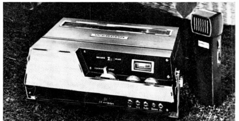
Webcor Rechargeable V—Model 2717: True music, voice reproduction at 1½, 3¾ speeds. Capstan drive, 5" reel. Operates on 5 rechargeable batteries (included), flashlight batteries or 110V, AC. Built in AC adaptor, battery charger. 5 input-output jacks, VU meter, battery charge indicator. Voice activated mike. Storage compartment holds AC cord, patch cord, earphone, batteries. Model 2715 same as above but with remote control dynamic mike.
