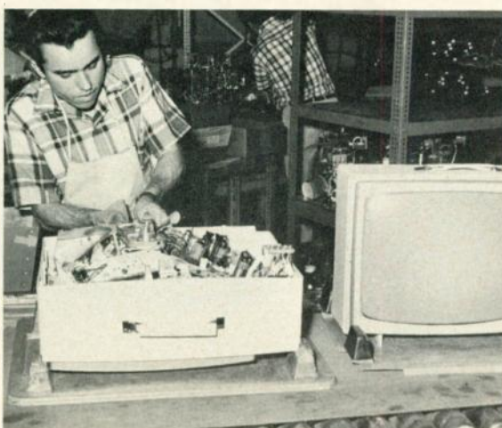
The final stage of chassis installation
