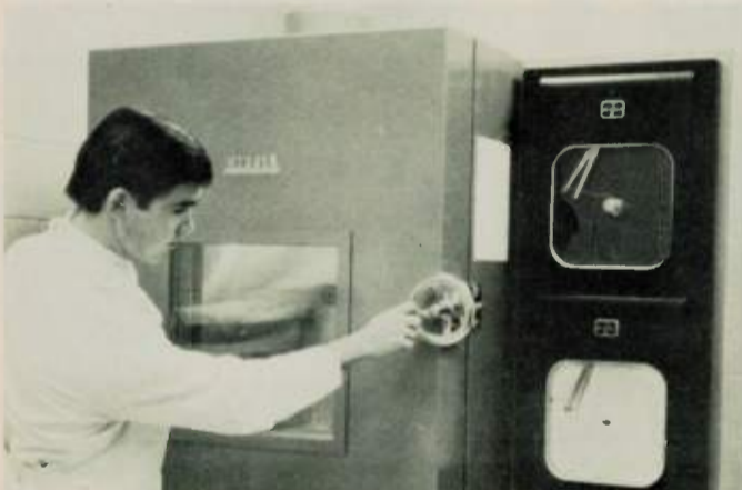
(4) To pass the temperature test, tapes must endure readings from 40 degrees below zero to 185 degrees in this chamber
