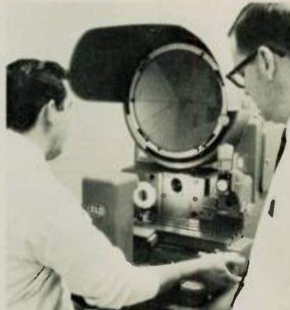
(5) This optical comparator checks track location to avoid cross-talk
