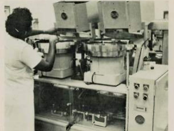
(6) RCA-developed automatic pinch roller sub-assembly machine puts a tire on the pinch roller hub
