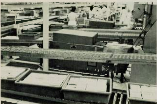
(7) In the packaging department, the finished cartridges are fitted into their specially designed plastic containers—some of them with 4-color labels—and moved in trays along the 4,000-ft. assembly line conveyor belt for a final round of inspection.
