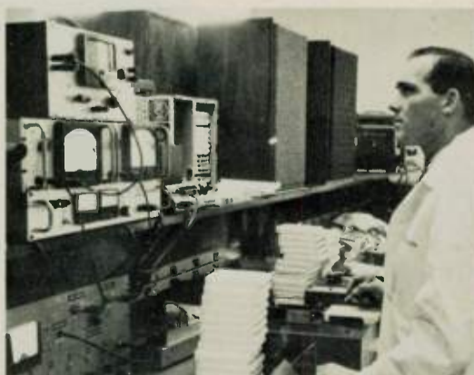
(8) The testing never stops at the Research and Development laboratory. Here, a special machine "listens" in a test to electronically detect "wow" and "flutter" on test tapes.
