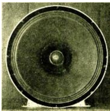
Showing the multiple-cone feature of the 18-inch dynamic speaker used with the Masterpiece V.
