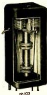
Another unusual feature for air dielectric condenser type intermediate-frequency transformers is that in the Miller DeLuxe series both primary and secondary circuits are adjustable from the top of the shield. The transformer is assembled in an aluminum shield 2" square and 4½" long, which is finished in fine black crackle Kem-Art baked enamel.
