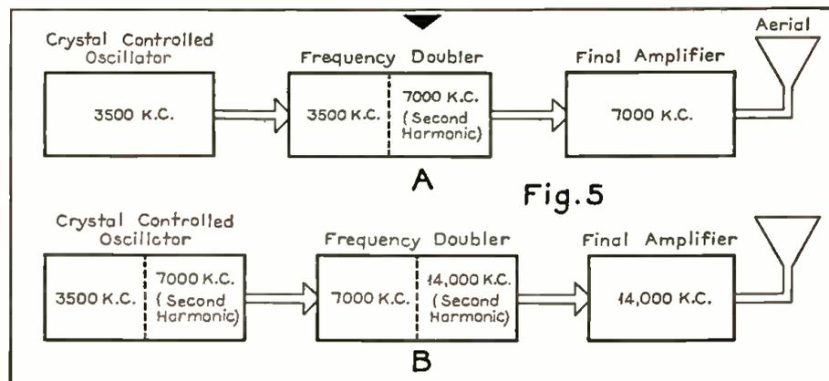
Block diagrams illustrating the manner in which a crystal-controlled transmitter can be operated in a number of bands with the same crystal.
