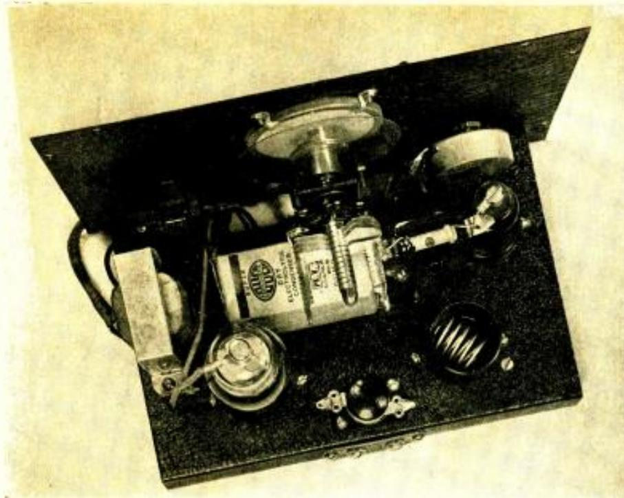
Above: Chassis view of the 5-meter receiver, showing location of parts. Below: The schematic diagram.
