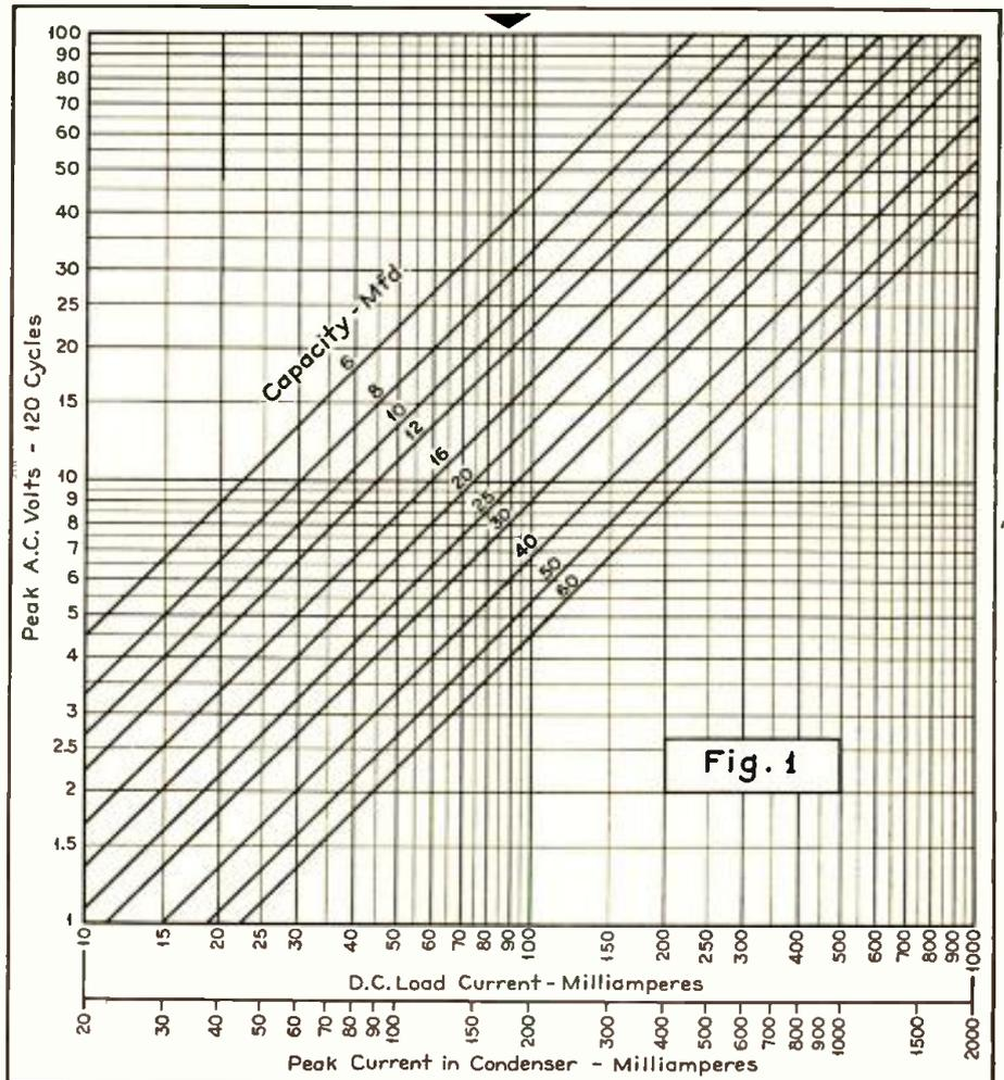
Chart from which may be determined the peak value of a ripple component for different values of load currents and input capacities. Based on use of full-wave 60-cycle rectifier; 120-cycle a.c. ripple.
