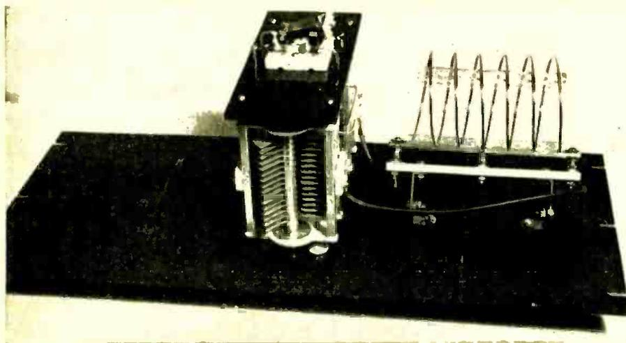
The AWR "Commercial" antenna tuning panel. Note series-parallel knife switch mounted on condenser ends.
