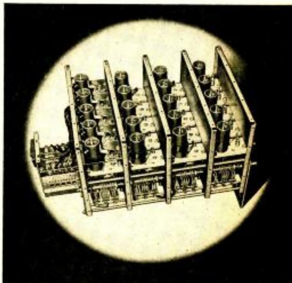
Fig. 3. View of the coil and condenser assembly comprising the heart of the r.f. section of the new Super-Pro. Note the gang of twelve band-spread condensers.
