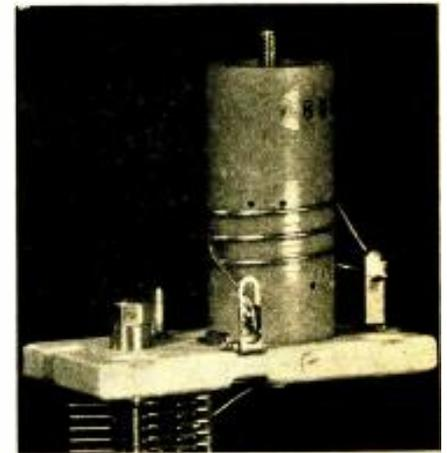
Fig. 4. The 20- to 40-mc. oscillator coil assembly. Note air trimmer below base and adjusting screw for copper tuning disc.
