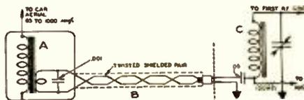
Energy in the antenna is impressed on the primary of Coil A where it is induced into the low-impedance secondary and fed into the matched line B, which is loaded with 1,000 mmfd. capacity at the input end.
