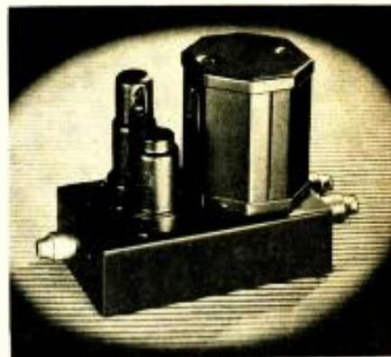
a 6F5 resistance coupled to a 6C5, providing 60 db gain. The input is high impedance and the output universal line impedances. Filtering is provided in the pre-amplifier to assure low hum level. If desired, a separate power supply can also be obtained for this unit. ALL-WAVE RADIO.
