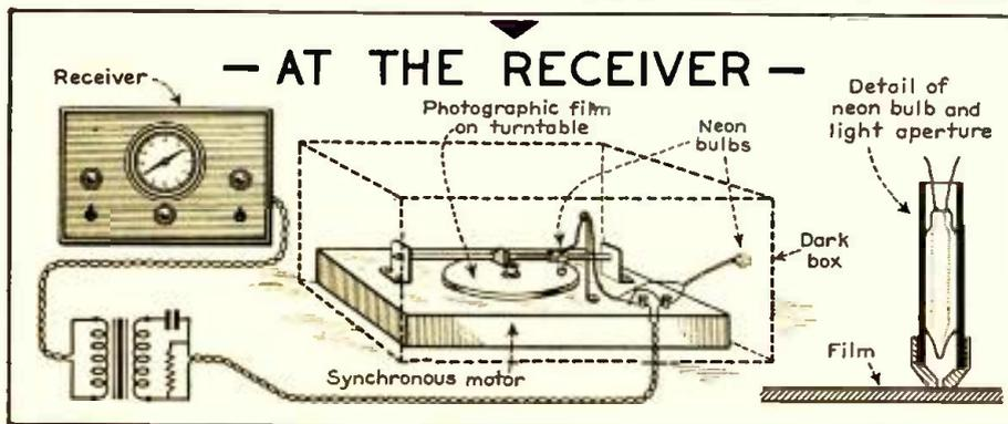
Experiments with this equipment have shown that pictures can be received at any distance providing the signal is strong and the motors synchronized. (Hints on handling of sensitive film, and film developing, by J. K. Thompson.)
