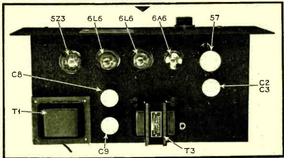
The complete speech amplifier. This is the top side view of the upper panel in the modulator unit. It incorporates a pair of 6L6 tubes in the output and delivers approximately 30 watts of Class A audio.
