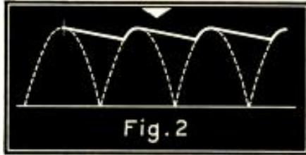
Illustrating a.c. ripple produced by repeated charge and discharge of input condenser.
