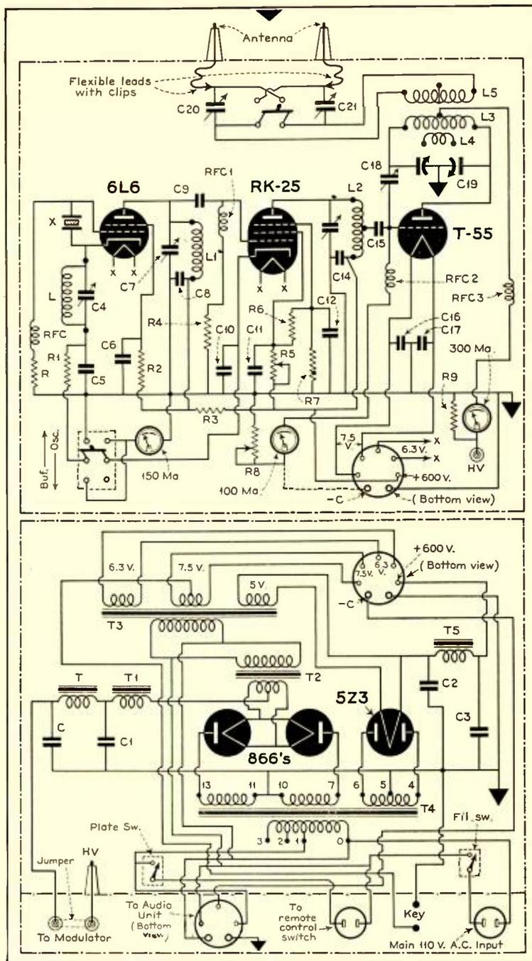
Complete schematic diagram of the c.w. section of the AWR "Commercial." Power supply unit at bottom, r.f. unit at top.
