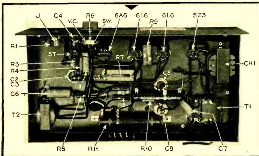
Under-panel view of the speech amplifier. Simplicity of design and neatness of construction are so apparent from this view that no further comment is necessary.
