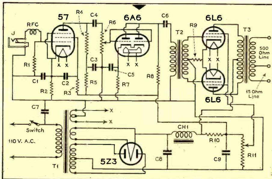
Complete schematic diagram of the speech amplifier for the "Flexible 400." The parts values are given in the list on this page.
