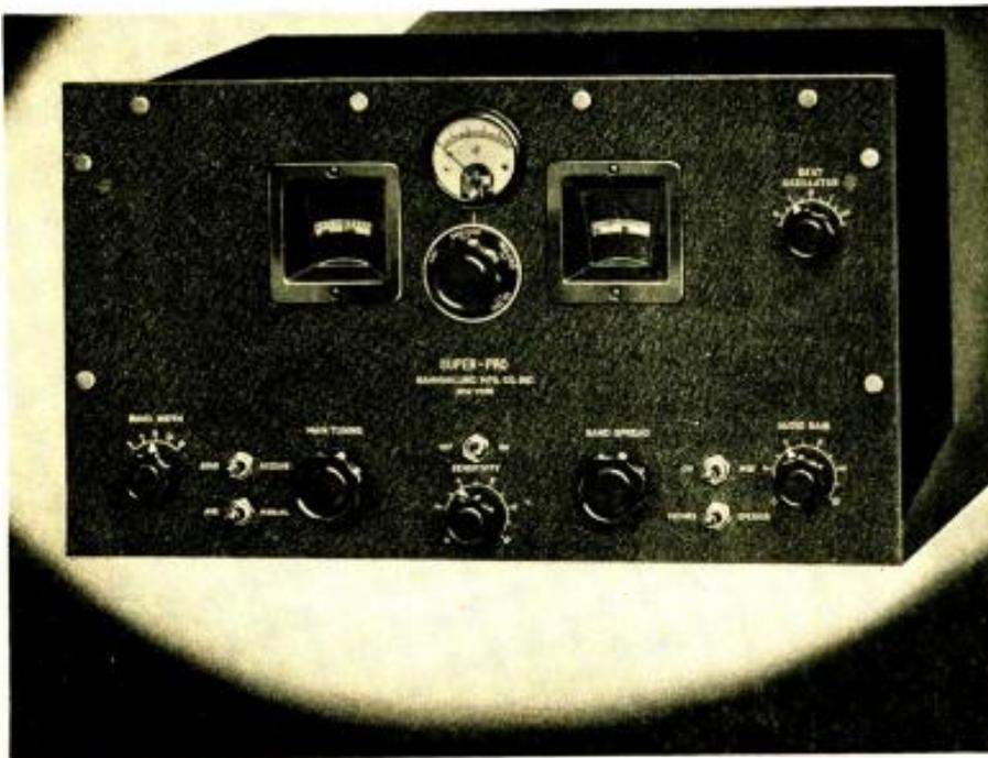
Fig. 1. Front-panel view of the new Hammarlund Super-Pro with calibrated manual controls. The band-width control has a range from 3 to 16 kc., and the beat-oscillator control from zero to 2500 cycles on either side of zero beat.
