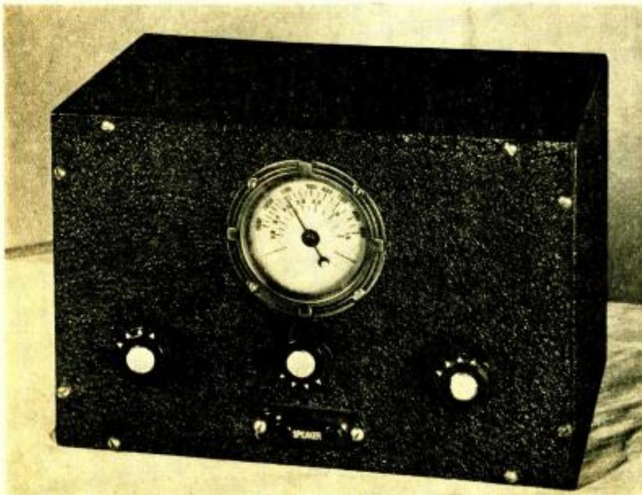
The midget a.c.-d.c. receiver designed for operation in the 5-meter band. By winding an additional coil, it will also make a good 10-meter receiver.
