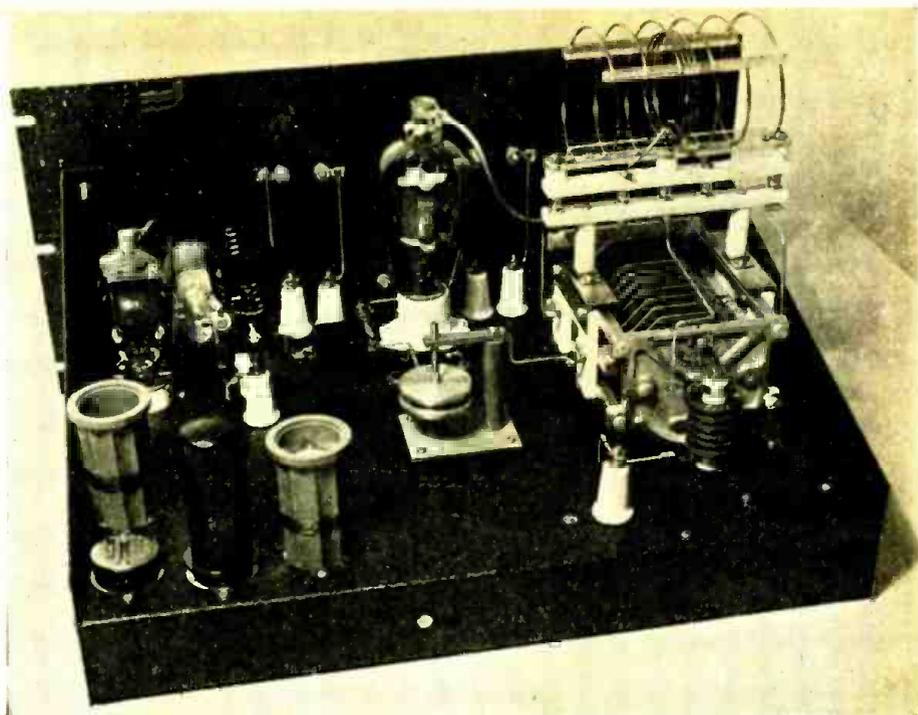
Rear view of the "Commercial" r.f. unit chassis. The T-55 tube and its neutralizing condenser, C18, are located in the center.
