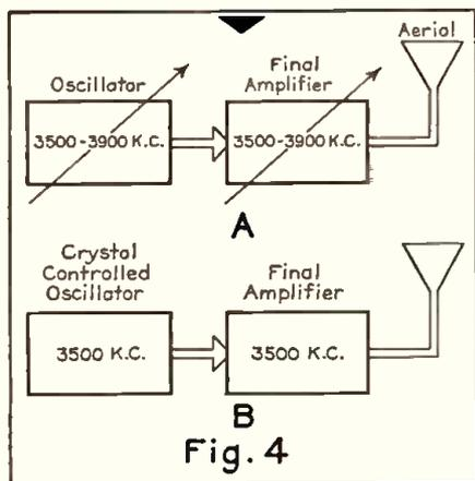
Block diagrams illustrating transmitters having variable-frequency and fixed-frequency tuning, the one at B being crystal controlled.
