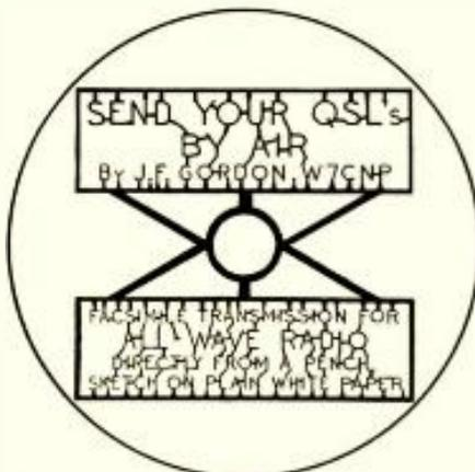
Fig. 1. The original drawing used in the transmission. The graphite conducting lines connecting the letters are covered with coil dope, and therefore are not transmitted, as can be seen from Fig. 2.
