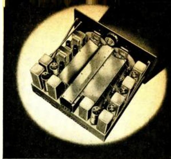
Fig. 2. Interior view of the new Super-Pro, showing where the metal tubes are located. Note that all units are enclosed and therefore protected from dust and damage.
