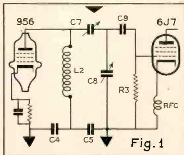
Fig. 1. The unique r.f. circuit used in the 5-and-10.
