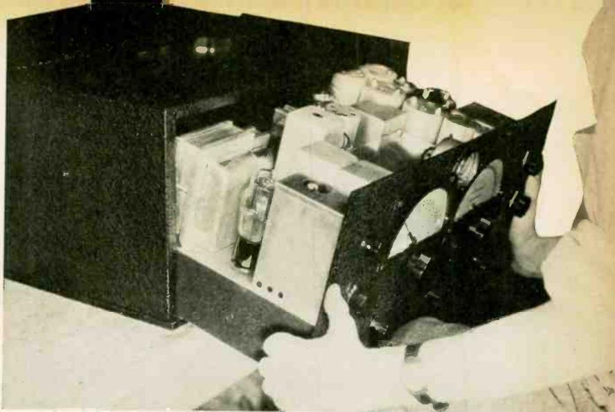
Pulling the RME chassis . . . note compact construction.
