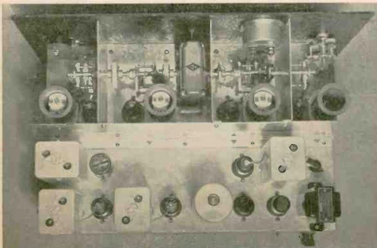
Looking into the chassis . . . note inter-stage shielding construction. The crystal "Transfilter" is directly behind the left metal tube at rear.
