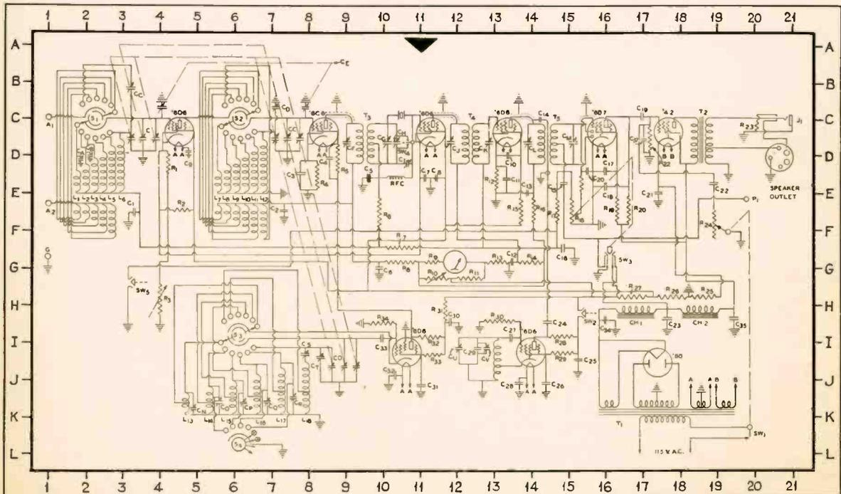
Fig. 1. The RME-69, less noise silencer, on paper, road-map style.
