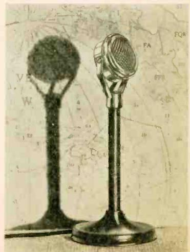
output signal quality from highly-selective receivers is greatly improved since the rising characteristic of the microphone tends to compensate for receiver side-band cutting.
