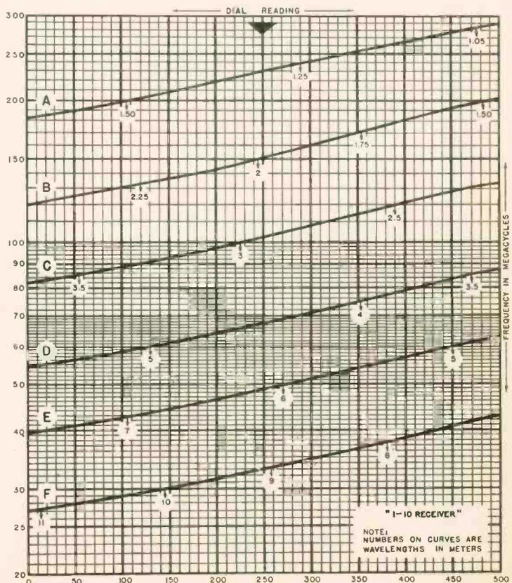
Fig. 2. The tuning range for each of the six sets of coils supplied with the "1-10" receiver.
