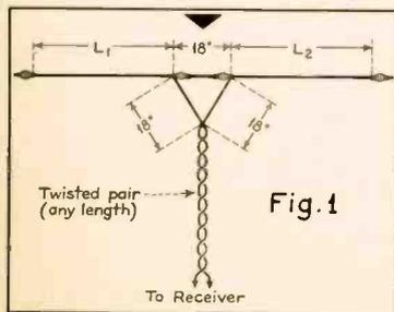
Illustrating the principles of antenna design for best results over a given frequency band.
