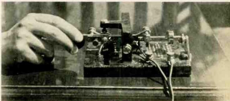
Fig. 2. Proper operation of a "bug" calls for a bit of physical nonchalance; too many beginners freeze at the key. Correct "stance" is illustrated in conjunction with one of McElroy's DeLuxe MacKeys.
