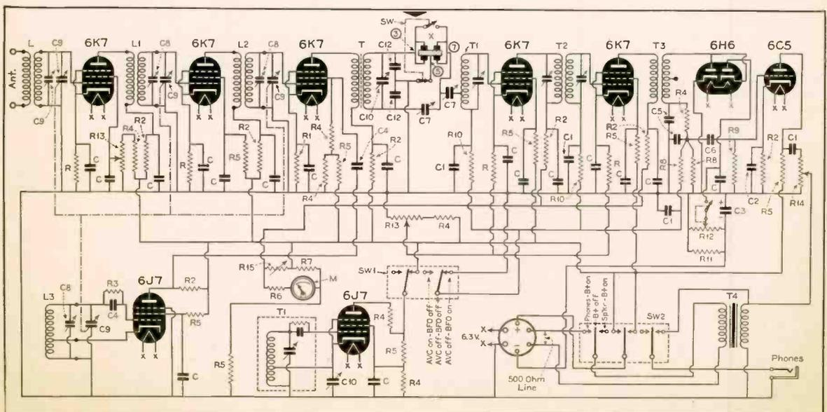
Schematic diagram of the receiver proper. Note crystal filter circuit.
