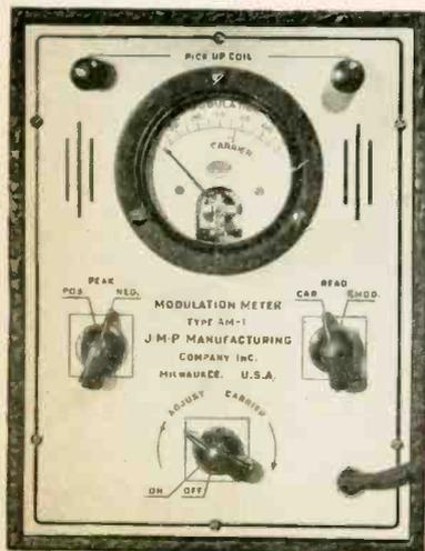
provided for positive or negative peak readings and for percentage modulation or carrier shift. It is designed to operate from a 115-volt a.c. or d.c. line.
