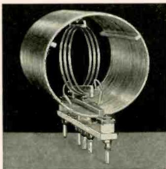
Variable link coupling is effected by pivoting a three-turn coil in the electrical center of the inductor, flexible pigtaills permitting rotation through 90 degrees. The pivot springs maintain a constant pressure on the link bearings, so that coupling adjustment will not be disturbed when changing bands. Fitted with steatite bar and five-contact plugs with phosphor bronze springs. ALL-WAVE RADIO.
