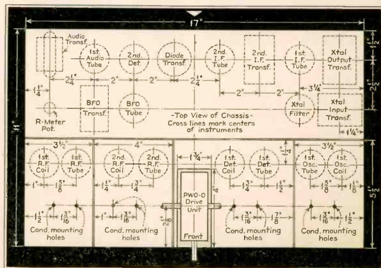
Working drawing of receiver chassis. This also indicates location of units.
