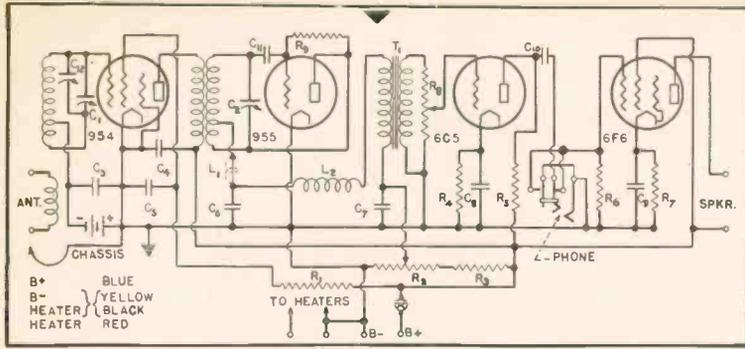
Fig. 1. The schematic diagram of the National "1-10" ultra-high-frequency receiver.
