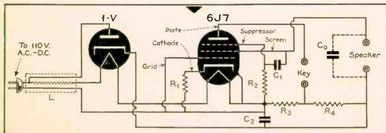
Here is the schematic diagram of the code-practice set. The 1-v tube is the rectifier and the 6J7 tube the oscillator. The filaments are in series with a resistance line cord, L, and operate directly from the power line. Tip jacks are used for the key and the loudspeaker, these being mounted on the front panel. Headphones may be used if desired.
