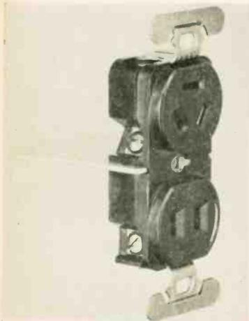
The slots in the radio side of the outlet for the ground and antenna circuit, and the prongs of the special cap are set at an angle not found in any other type of convenience outlet. The special cap cannot be used with any other outlet. ALL-WAVE RADIO.
