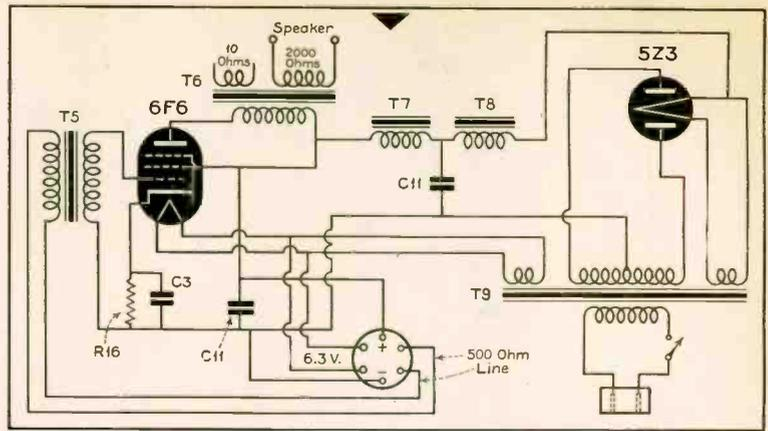
Schematic diagram of power amplifier and power-supply unit.
