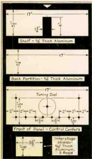
Details of front panel and shield partitions for 2TP's superhet.
