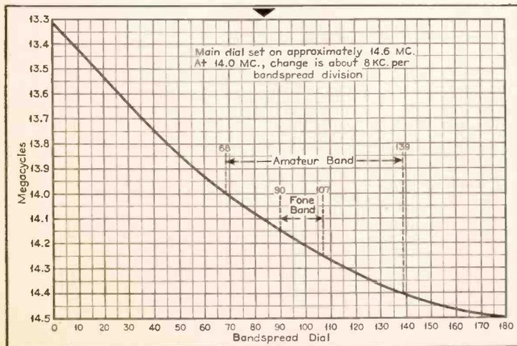
Fig. 2. Bandsread tuning in the 14-megacycle region.
