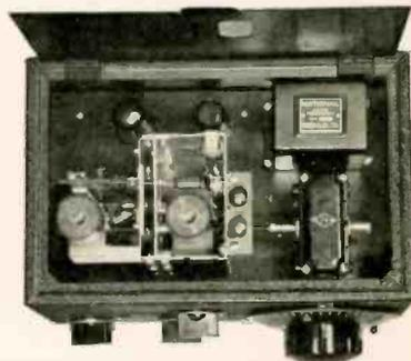
Interior view of National "1-10" showing integrated r.f. unit. Note small, enclosed plug-in coils.
