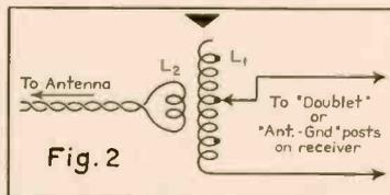
Link coupling to the receiver when the receiver input does not match the impedance of the twisted transmission line.
