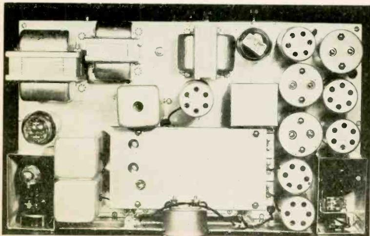
Looking down on the RME chassis. Main and bandsread tuning condensers are contained in central, shielded compartment.
