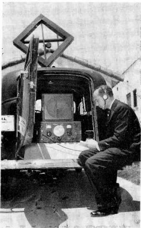
*F.C.C. "Police Patrol" equipped with Hallcrafters SX-17 Super Sky rider. Several of these scout cars are in daily use, trapping "bootleggers" and checking other transmissions. Recordings of broadcast programs are also made and sent to Washington for checking purposes.*
