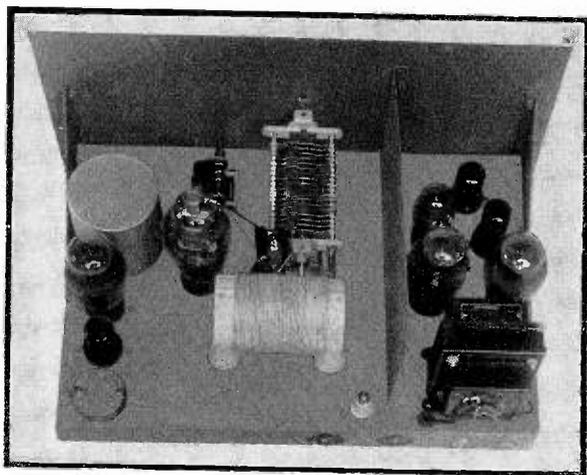
*R-F and Audio Components for the 812 Grid-Neutralized Transmitter. Note shield plate between audio and r-f stages.*
