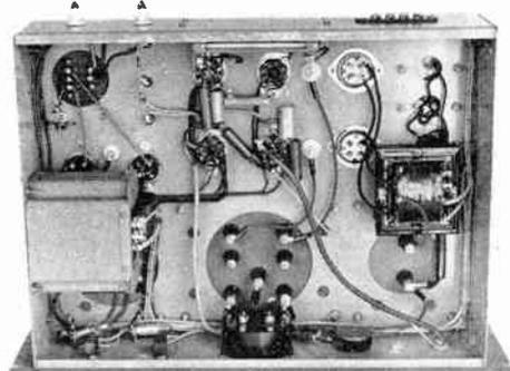
*Top and bottom views of exciter, showing Thordarson dual-voltage power transformer and dual rectifier components. This deck is a complete c.w. transmitter, power supply and all.*
