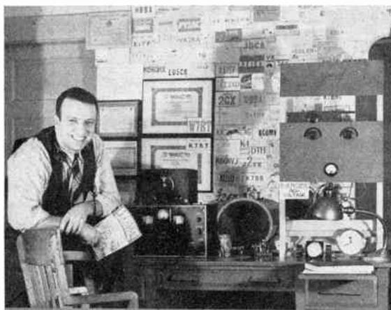
• Here's the operating spot at W7RT. Equipment includes HQ120-X receiver with home-made preselector, and an auxiliary receiver in the SW3 atop the HQ120-X. Transmitter is an 811 final with 150 watts on 40 and 20 c.w. Note two WAC certifs—from two locations, first in Seattle, and next in Goodnews Bay, Alaska, as K7RT.
