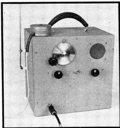
*The complete 2½-Meter Transceiver in a deluxe carrying case which has ample space for holding the A-, B-, and C-batteries. The microphone is a standard Western Electric F-1 unit, in a special housing.*
