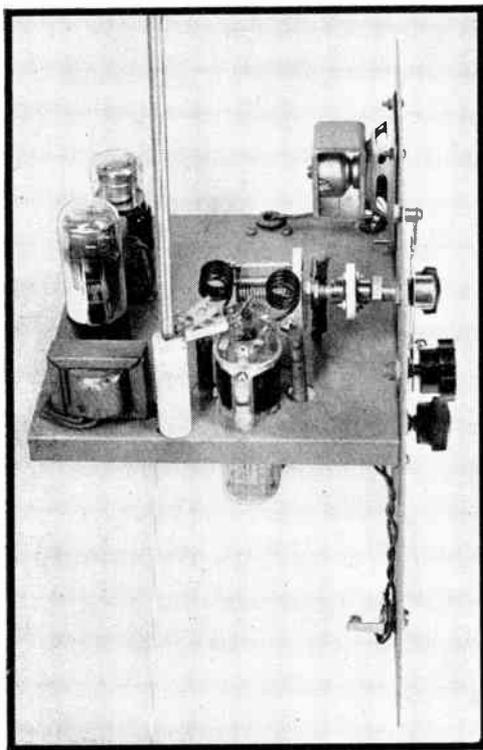
*The transceiver should be thoroughly tested before it is installed in its carrying case. A temporary antenna-rod assembly is illustrated in the photograph above.*
