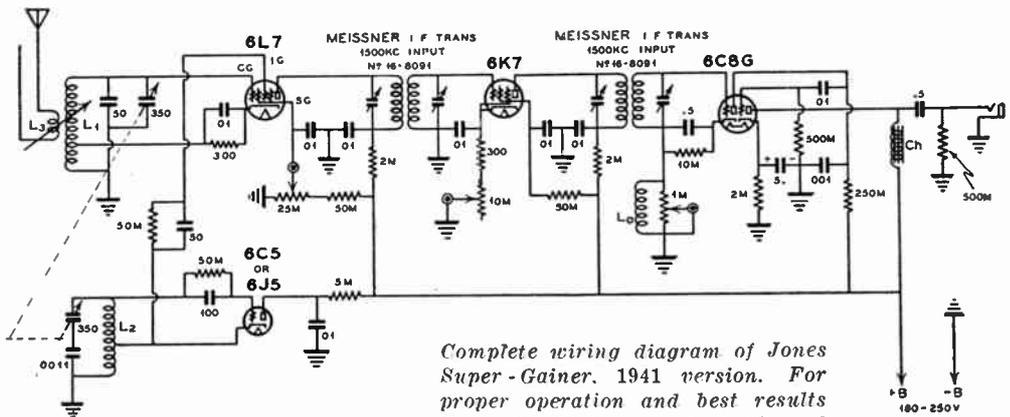
Complete wiring diagram of Jones Super-Gainer, 1941 version. For proper operation and best results there should be no substitution of circuit components.
