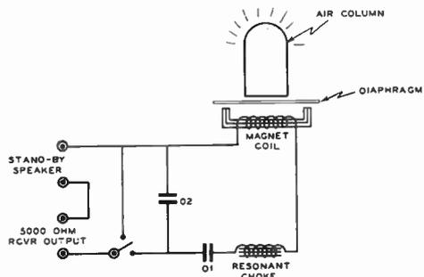
Complete circuit of the Uni-Signal Selector for conventional operation.
