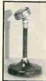
Double your power with VT-73, built especially for voice transmission. Speech frequencies emphasized by creating a rising curvature of response between 500 and 4,000 cycles. Crisp, clear signals, even through QRM. Combination microphone, handle and stand, weighs 27 ounces. Anti-resonant cable. Climatically sealed. Fully R.F. shielded. Won't blast from close speaking. High output -50DB. Finished
