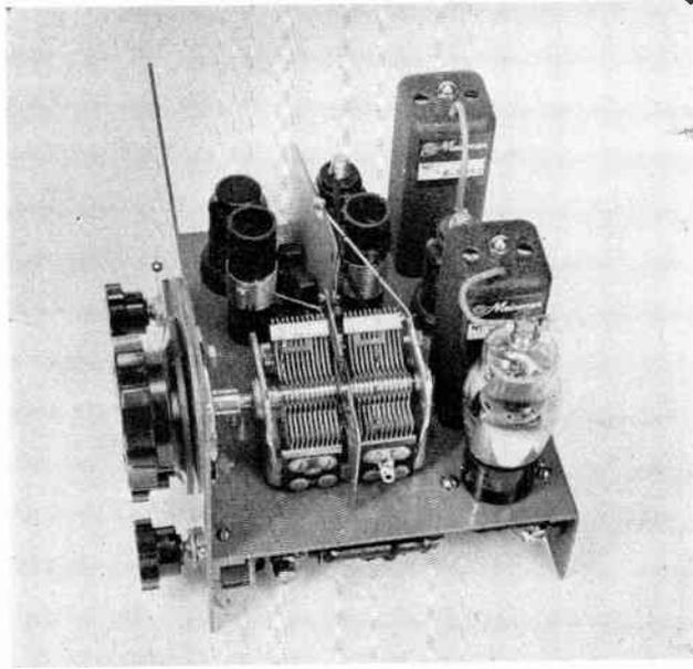
Looking into the Super-Gainer, all above-chassis components are clearly shown. The shield plate between the coils is grounded to the frame of the main tuning condenser. The 1,500-Kc. i.f. transformers are of the Meissner Mfg. Co. type, the catalog numbers being shown in the schematic wiring diagram.
