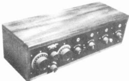
**MODEL XJ** - The TRF Model XJ four tube receiver was also offered as a regenerative version and called the "SJ-Super". The only identifiable difference on the panel is the push-pull regeneration coil control knob above the tap switches between the two tuning dials. Very few of these sets are around.
