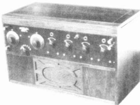
**MODEL XV** - The Model XV (fifteen) was in reality the Model X in a deluxe cabinet that contained a speaker chamber with a wood horn (no driver) and space for batteries. Access to the set was from the top lid and door panel in the rear. In 1923 it sold for \$70 without tubes, batteries, or antenna. Complete cost was \$127. A similar, but slightly smaller cabinet was sold to house the Crosley VI (six) and was called the Model XII. It sold for \$5 less.
