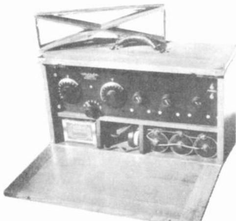
**MODEL VIII-P** - The Model VIII was sold in a handsome oak portable case that held batteries and phones and antenna wire holder. Its price without the extras was \$60. Adapters were needed to use dry-cell tubes in the porcelain sockets. Its sister set the Model VI (six) also came in an oak portable case for \$40.
