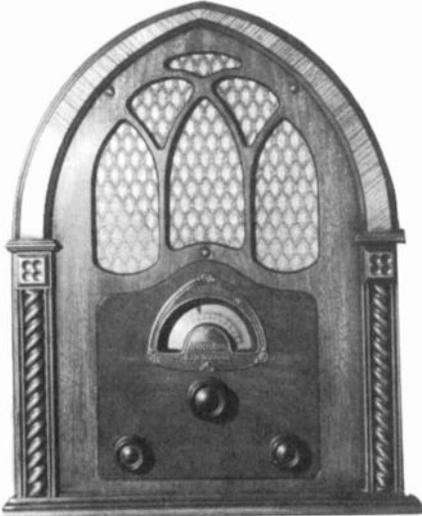
**ATWATER KENT** - Model 82, it is a seven tube superhet using two 35's, one 27, two 24's, one 47 and one 80 tubes. Made in 1931, it sold for \$69.80 with tubes. (Karl Rommel - Lansing, MI)
