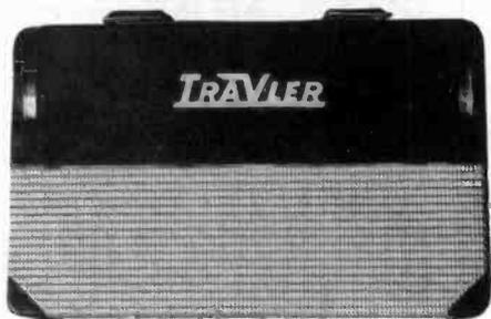
**TRAVLER MODEL 5300** - A four-tube, battery-operated, plastic, portable AM radio with formed grille cloth, this 1950s unit has all four original Traver tubes. (*Larry Mitchell - Denver, CO*)
