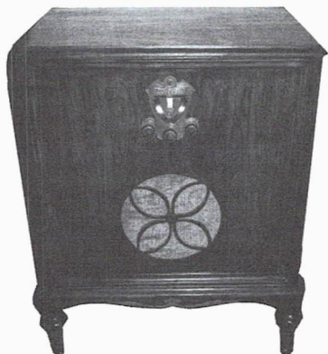
RCA VICTOR 28 - I am new to the hobby, and this is my first restoration. The cabinet was very poor, and the radio did not work. I brought the radio to life after a month's work, and a friend replaced the top veneer. The rest of the cabinet is original. (R. Morrison - Comox, B.C., Canada)
