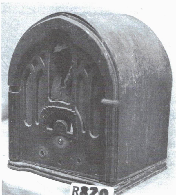
Figure 1. The Knight cathedral in found condition with the case in three parts — bottom, front and top/sides.
