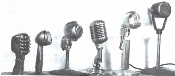
Figure 7. These early vintage microphones are from left to right: Electro-Voice Mercury Model 611, Astatic Model VHD, Turner Model 22D, Shure Unidene 55-S, Turner Model 33D and Turner Model U9S.
