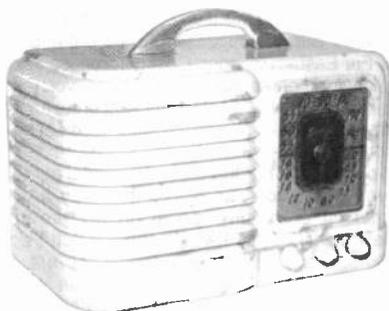
**SENTINEL MODEL 212** – Listed in Rider's, Volume 12, page 1, this 6-tube Art Deco radio has a white plastic (Plaskon or urea?) cabinet with beautiful green and rust marbling. It operates on shortwave frequencies of 5.7 to 18.3 MHz, as well as the broadcast band. Dimensions are 12" x 8" x 7". (Merrill Mabbs – Rapid City, SD)
