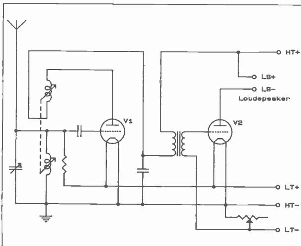
Figure 2. The circuit design of the Ethophone Duplex.
