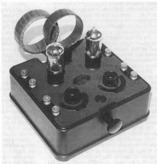
Figure 1. The Burndept Ethophone Duplex 2-valve receiver, shown here with two Mullard D.06 type valves.
