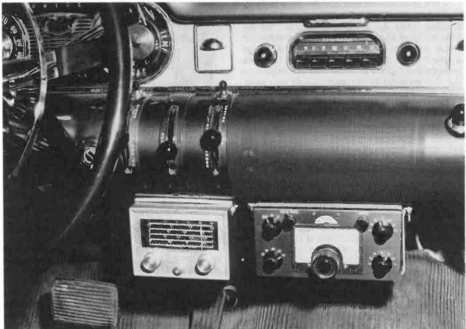
Figure 1. A pre-production Palco Bantam mounted under the dash of a 1954 Buick automobile. At left is a Morrow Model 5BR series converter.
