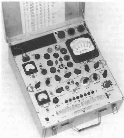
Figure 2. The Western Electric Model KS-15750-L1 tube tester manufactured by Hickok.
