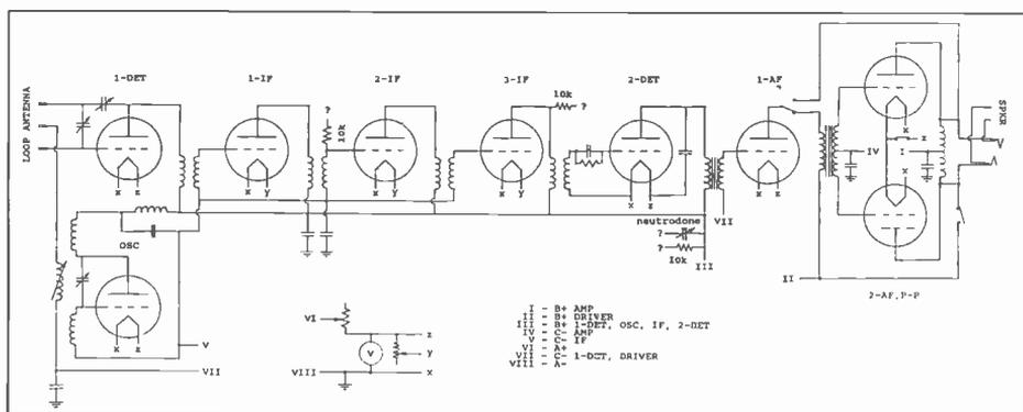
Figure 4. The shop-built superheterodyne schematic.
