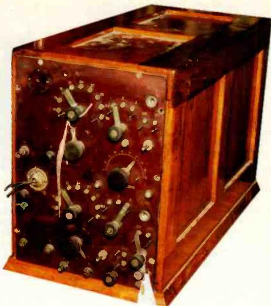
*This 1914 DeForest 2-step amplifier, missing the two spherical audions and sockets, sold for \$27,500. (Terrey photo)*
