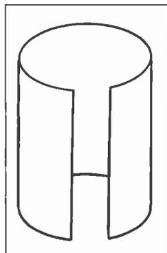
Figure 2. The cylindrical-shaped paper diaphragm of the DeForest Audalton.
