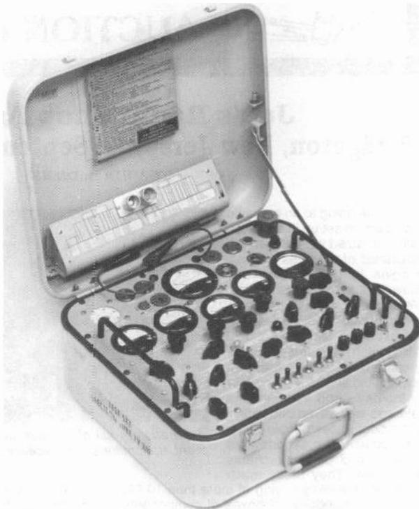
Figure 3. The Model TV-2/U military tube tester manufactured by Hickok. Notice the tube pin straighteners mounted above the roll chart.
