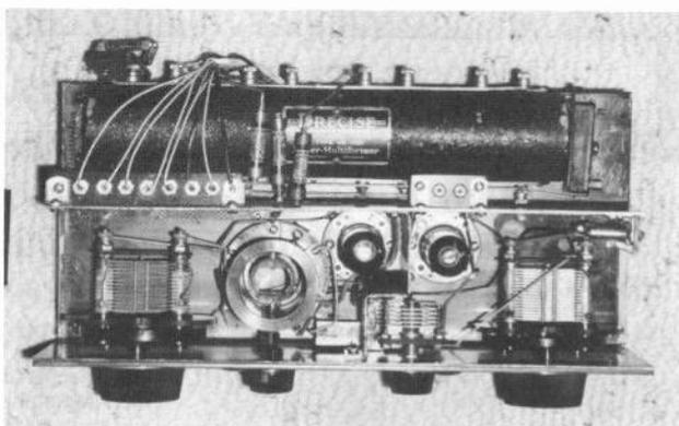
Figure 3. Bottom view showing the shielded first detector and oscillator stages.
