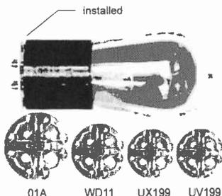
These tube repair wafers are solid-state devices for quick and easy repair of early vacuum tubes. The wafer is installed by simply sliding it over the tube pins and reinserting the tube into its socket. If the filament is intact, but there is little or no emission, the filament may be lit for best visual effect. However, the tube can be open filament.
