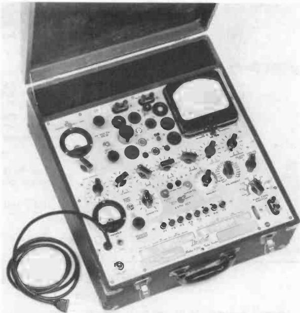
Figure 1. The Hickok Model 539C tube tester.
