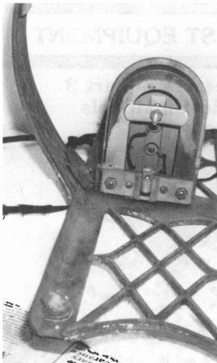
Figure 4. Rear view of the electromagnetic driver showing the mechanism and horseshoe magnet.
