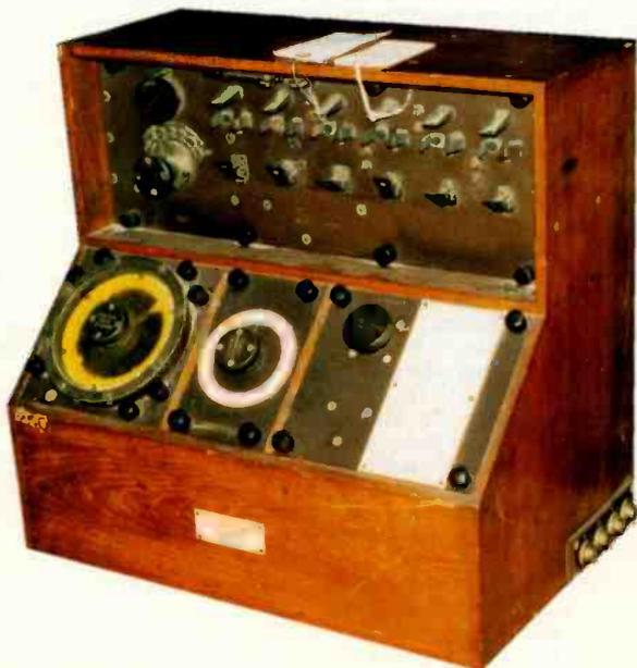
*This British Marconi Type 11 DF direction finding receiver sold for \$9,000, less the six V24 tubes. (Terrey photo)*
