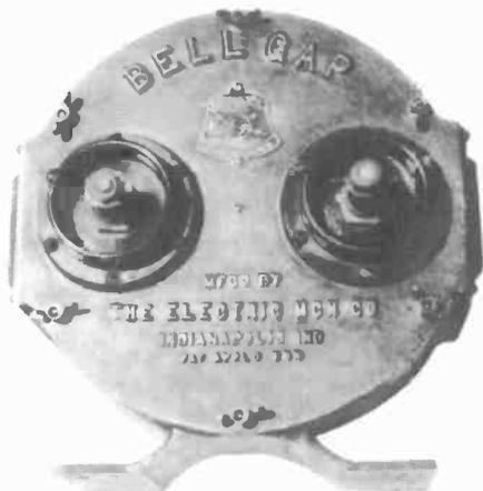
**BELL GAP** – Manufactured by the Electric Machine Co. of Indianapolis, Indiana, this rotary spark gap, ca. 1920, has an aluminum housing. (Larry Chestnut – Ellington, CT)
