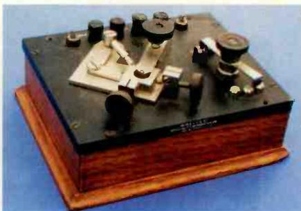
*This Wireless Specialty Apparatus IP-175 silicon detector was one of the many crystal detectors offered. (Terrey photo)*
