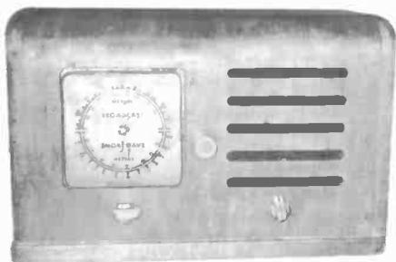
**INDUSTRIAL TOOL AND DIE MODEL W6T2B** – Of the 150 radios in my collection, I think this is the oddball. The cabinet has a blonde finish. The chassis has 6 tubes with AC/DC, broadcast and shortwave. (Vernon Blaine – Canby, MN)
