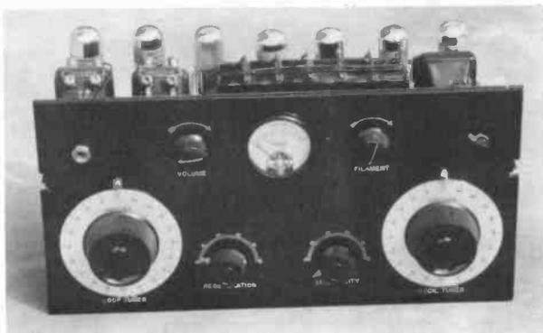
Figure 1. The shop-built superheterodyne. Two additional tubes are located under the chassis.
