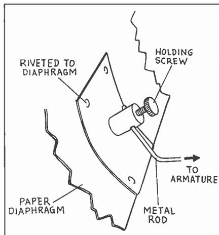
Figure 3. The mechanical linkage between the diaphragm and the armature.
