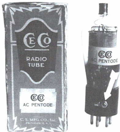
Figure 2. A CeCo Type P1 tube and its carton. The arrow points to a tube base connection for the "space-charge" grid.
