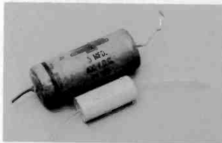
Figure 11. Modern capacitors with plastic film dielectric are much smaller than the old paper dielectric capacitors.
