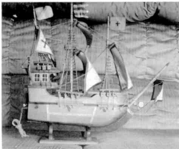
Figure 1. The wooden ship model that in reality is a radio antenna.
