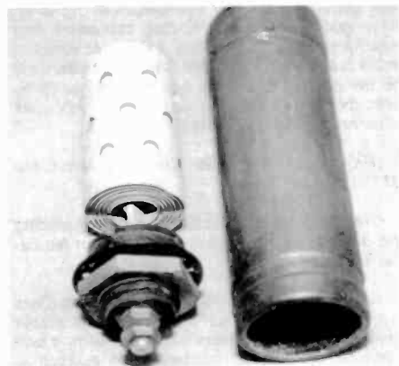
Figure 8. A copper, can-type, wet electrolytic capacitor from a Philco radio.
