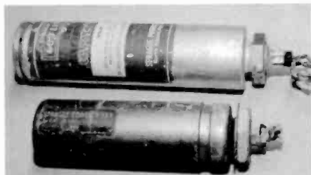
Figure 6. Two examples of can-type electrolytic capacitors: a wet type at the bottom and a dry type at the top. Note the nut and threaded base used to mount the capacitors.
