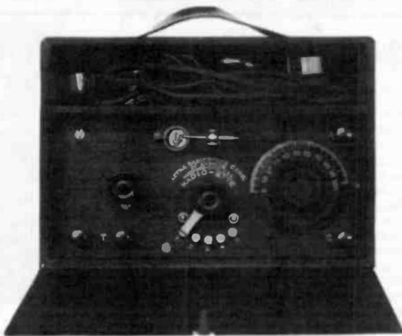
Figure 1. The portable Aetna crystal set with its handle showing and cover down. Seen at the top of the panel is the crystal detector. Under it are the words: "AETNA RADIOPHONE CORP. OF AMERICA, HARTFORD—CONN. U.S.A., RADIO-ETTE." The set has binding posts for antenna, ground, and headphones.
