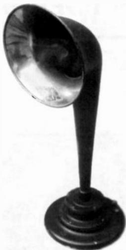
**TMC HORN SPEAKER** - This small metal horn with wooden base was made in England by the Telephone Mfg. Co. TMC on the nameplate is defined as "TrueMusiC." It is 18" tall with a 6" wide bell that is electroplated copper inside. (Dave Crocker - Mashpee, MA)
