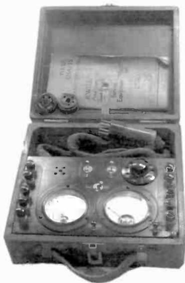
**WESTON MODEL 537 SET ANALYZER** – This 1920s vintage analyzer was used to test radio circuitry. The tester enabled the serviceman to measure filament, grid bias and plate voltages, as well as cathode and plate currents. Included are adapters for 4- and 5-pin tubes, such as 171-A, 226, 227, 245, 280, and 281. (Paul Jachim – Indian Head Park, IL)
