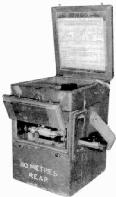
**BRITISH ARMY TRANSMITTER** – The British Army used this portable spark transmitter, ca. 1917, in the trenches of World War I. The photo shows the door open exposing the adjustable spark gap, while on the right is the integral code key. (*Jim Taylor – Bournemouth, England*)
