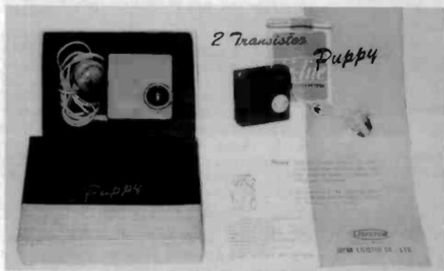
**"PUPPY" TRANSISTOR RADIO** – Manufactured by the Japan Lisistor Co., Ltd., this 2-transistor receiver was advertised as the smallest transistor radio in the world, weighing a mere 40 grams. Inside is a flat-type mercury battery. The plastic case came in either red, green, or tan, and it is shown here in its presentation box containing the earphone. (Erwin Macho – Vienna, Austria)
