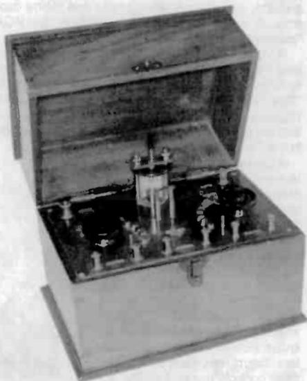
**REFLEX CRYSTAL RADIO** – Manufactured in the early 1920s by the Reflex Radio Co., this British receiver has a glass-enclosed crystal detector. The hardware is all gold-plated. (Jim Taylor – Bournemouth, England)
