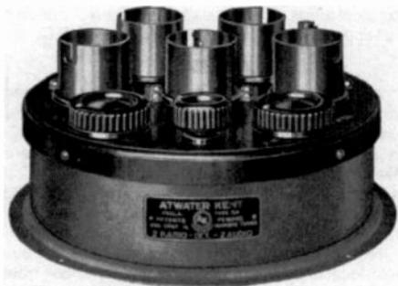
Figure 2. The 5-tube TA unit (Type 4330) used on the Model 8.
