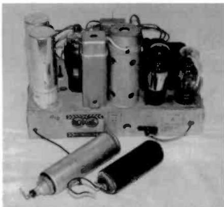
Figure 2. The compact chassis of this "4-tuber" is shown with new filter capacitors in place. The two capacitors in front of the chassis are the bad units.
