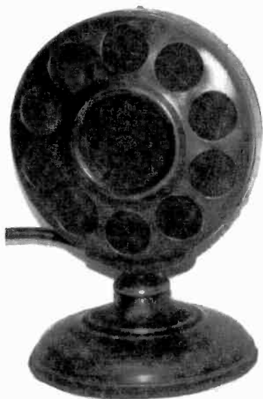
WESTERN ELECTRIC MICROPHONE – This table microphone was one of the more widely used types of the mid-1920s and early 1930s. It has a double button pickup which is spring-mounted inside. ( Wally Worth – Wollaston, MA )
