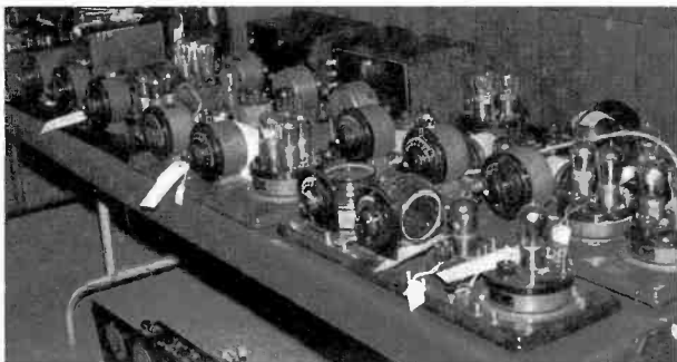
This great selection of Atwater Kent breadboards included some early models, along with Models 9, 10 and 12.
