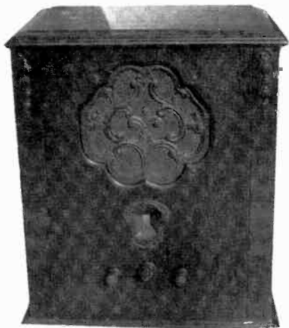
KOLSTER MODEL K-60 – This 7-tube tombstone, with a decorative Repwood-type grille, was manufactured in 1931 by the Federal Telegraph Co. of New York. This company had no connection with the Federal Telephone and Telegraph Co. of Buffalo. ( Dave Crocker – Mashpee, MA )
