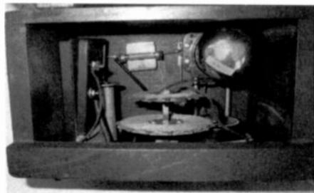
Figure 2. Looking down into the interior of the Crosley Model 50, showing the patented book-type tuning condenser and the operating cam shaft at the left.
