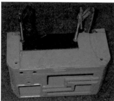
Figure 2. A replacement piece of Bakelite is clamped in place in preparation for gluing.
